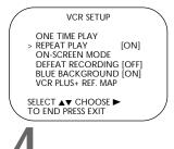
**Press the STATUS/EXIT button.** Now, when a tape has finished playing, the TV/VCR will rewind it and start playback again. (TV programming will appear while the tape is rewinding.)
